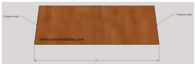
**Step 3.** Cut the Short Sides. Cut 2 pieces of 1×4 to 6-9/16", then cut a 5 degree angle on each end. Drill pocket holes in each end and one pocket hole in the top (shorter side). These pocket holes will be used to attach the top in Step 10.
