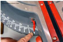
**1b.** Set miter saw bevel to 5 degrees.
