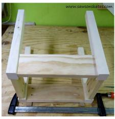
**Step 7.** Cut the Top pieces. Cut 3 pieces of 2×4 to 15". On 2 pieces, mark 1/2" on 2 corners and cut a 45 degree angle.
