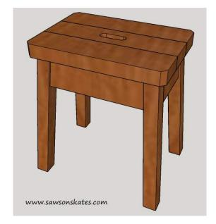
**Step 1**. Cut Legs. Set miter saw table to 5 degrees. Set miter saw bevel to 5 degrees. Cut first angle on 2×2. Leave piece on the saw. Measure from the miter you just cut, along the top of the piece and make a mark at 16-1/8". Slide the piece, so the mark corresponds with the saw blade. Place a stop at the end of the piece, so you can cut the other three legs to the same length. Make your cut and repeat for the other three legs.
