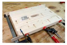
**Step 10.** Attach top to legs. Place the top on your workbench, so you are looking at the bottom. Center legs on the top, clamp and attach using 1-1/4" pocket screws.
