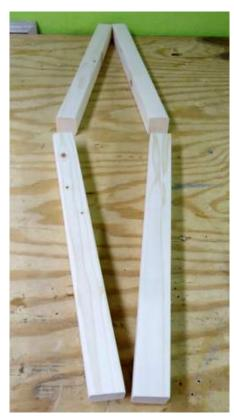
**Step 5.** Attach Short Sides. With the top of the legs still facing you, put two pieces of scrap 1/4" material on the workbench in between the legs. This scrap will set the side in 1/4". Apply glue to each end of a Short Side, place between legs (so the short edge is facing towards you) on top of the scrap, clamp to the legs and attach using 1-1/4" pocket screws. Repeat with the other set of legs and Short Side.
