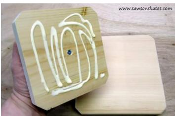
**Step 12.** Cut the Stopper. Measure the inside dimensions of the container and deduct an 1/8" from each dimension. Cut a piece of wood to this dimension to form a stopper for the neck of the container. Drill a few countersink holes in the stopper. Apply glue to the stopper, center on the bottom of the top and attach using 1-1/4" wood screws.
