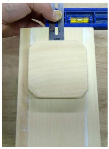
**Step 9**. Attach the Nozzles. Apply glue to the nozzle, center on the nozzle base and attach using 1-1/4" finish nails. Repeat for the other two sides.
