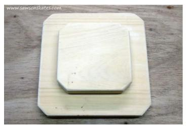
**Step 13 continued.** Attach medium top to small top using 1-1/4 wood screws. Apply glue to the medium top, center the large top (Step 11) and attach using 1-1/4 wood screws.
