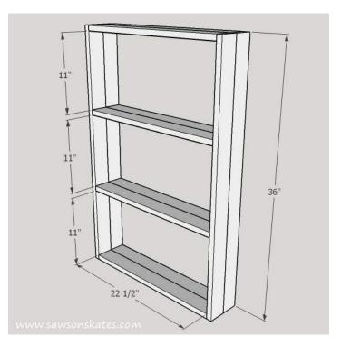
**Step 3.** Assemble the Shelves. Take 4 of the shelf boards and drill three pocket holes in the edges. Clamp one board with pocket holes to one board without pocket holes and attach using 1-1/4" pocket screws. Repeat for remaining boards.
