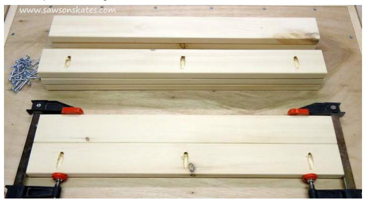
Step 4. After the shelves are assembled, drill two pocket holes in each end of the shelves.
