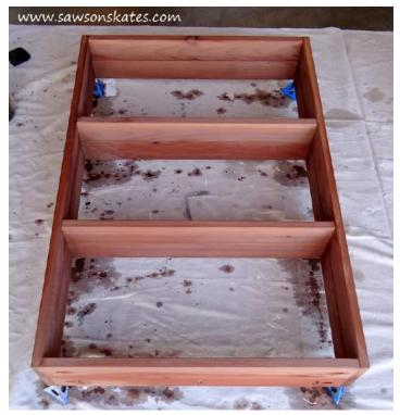
**Step 8.** Attach the Back. Cut the back to 36". Apply painter's tape on the cut line to avoid chipping the chalkboard. For an easy way to make a long straight cut, check out my "How to Make Circular Saw Crosscut Jig". I applied some of the Kona stain I used for the shelf to the edge of the chalkboard, so it would blend with the shelf. Clamp the back in position and attach using 1-1/4" finish nails.
