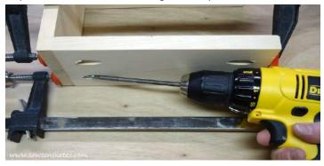
**Step 11.** Attach the Right Side. Apply glue to the top and bottom, clamp side in position and attach using 1-1/4" pocket screws. Attach right side shelf and middle shelf using 1-1/4" finish nails.
