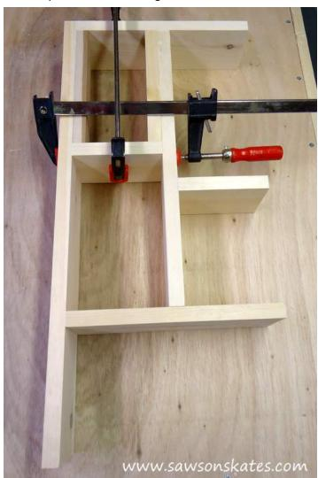
**Step 10.** Attach Bottom. Apply glue to bottom, clamp in position and attach using 1-1/4" pocket screws.
