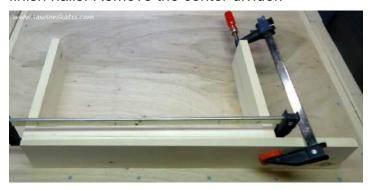
**Step 6.** Cut the Small Shelves. Cut 3 pieces of 1×4 to 4-13/16". 2 will be used as shelves and 1 will be used to help properly align the center divider.
