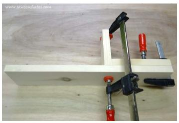
**Step 8.** Attach Center Divider. Insert two of the small shelves (from Step 6) and use them as spacers on the left side (do not attach), apply glue to the center divider, place in position and attach using 1-1/4" finish nails. Remove the spacer shelves.
