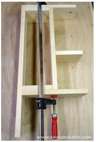
**Step 9.** Attach the Left Shelf. Cut 2 pieces of scrap to 7-11/16". Place the scrap against the top shelf, insert one of the spacer shelves from Step 8, clamp and attach using 1-1/4" finish nails.
