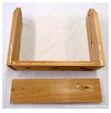
**Step 6.** continued... Replace the front making sure the sides and bottom are flush and attach using 1-1/4" finish nails. Repeat for the back.
