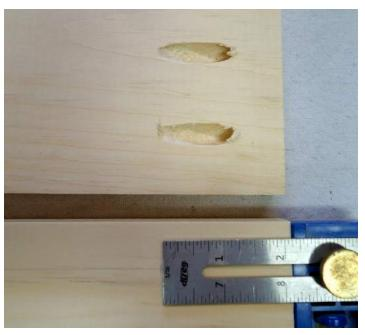
**Step 3.** Assemble the Tray. Place the sides so the countersink holes face inward and are at the top of the boards. Clamp sides together, check for square and attach using 1-1/4" pocket screws.
