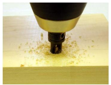
Step 2. Cut the Short Sides of the Tray. Cut 2 pieces of 1×4 to 12-1/2". Drill pocket holes in each end. On the opposite side of the pocket holes, Layout the countersink holes to attach the sides to the opening. Set the Kreg Multi-Mark to 3/4" and draw a faint line on one edge. Measure in about 2-1/8" (to avoid drilling into the pocket holes) on each side and make a mark. Also make a mark at the middle. Drill a countersink hole at each location.
