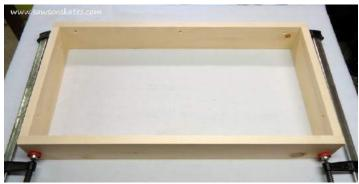
**Step 4.** Cut the Tray Bottom. Flip the tray so the countersink holes are now at the bottom. The tray bottom should measure 27" x 14", but it's a good idea to measure the sides and adjust if necessary. Place the bottom on the tray sides. Set the Kreg Multi-Mark to 3/8" and draw a faint line around the edge of the bottom. Drill countersink holes on the line and attach bottom to the sides using 1-1/4" wood screws.
