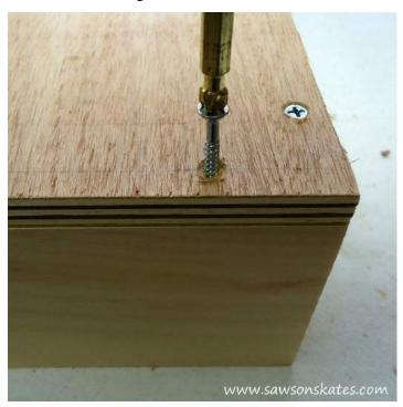
**Step 5.** Install the Tray. I placed some scrap wood on the floor equal to the distance from the floor to the bottom of the tray to help properly position the tray. Slide the tray in position and attach using 1-1/4" wood screws.
