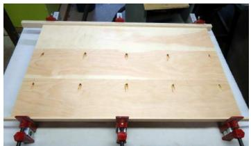
**Step 11.** Attach the Top. Place the top on the cabinet with the back of the top flush with the back of the cabinet and center top side to side on the cabinet. Clamp the top to the cabinet and attach using 1-1/4" pocket screws. Drill a few countersink holes in the bottom of the back brace and attach using 2" wood screws.
