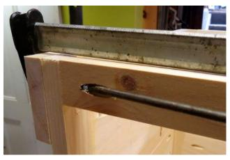
**Step 10.** Make the Top. Cut 3 pieces of 1×8 to 28" and rip to 5-3/4". Drill pocket holes in the edge of 2 pieces. Clamp pieces and attach using 1-1/4" pocket screws.
