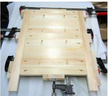
**Step 7.** (continued) On the back (same side as the other pocket holes) drill pocket holes in the top of each stile and the middle of the rail. These pocket holes will be used to attach the side to the top. Also drill 3 pocket holes in the front stile. These pocket holes will be used to attach the side to the front. Be sure to make a right and left side panel. Repeat Step 7 for the second side.
