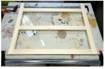
With the drawer fronts removed, roundover the drawer openings. Just like rounding over the drawer fronts, this will give the illusion that it's an actual drawer.
