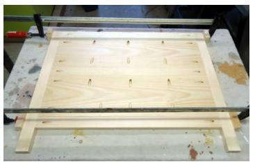
Flip the assembly to the front side and gently remove the drawer fronts.
