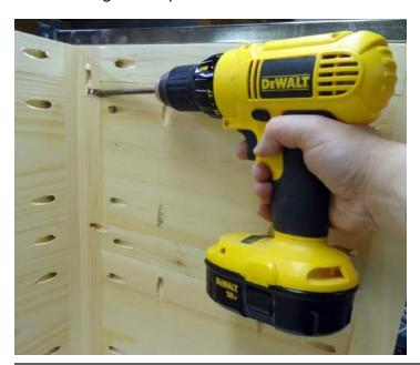
**Step 9.** Cut and Install the Back Brace. Cut a 1×2 to 25-1/4" and drill a pocket hole in each end. Clamp at the top of the sides and attach using 1-1/4" pocket screws.
