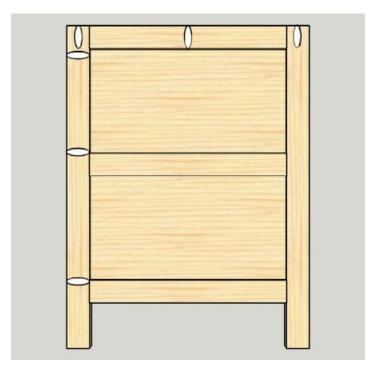
**Step 8.** Attach the Sides to the Front. Clamp the side to the front making sure the pocket hole screws in the side stiles face the front assembly. Attach using 1-1/4" pocket screws.
