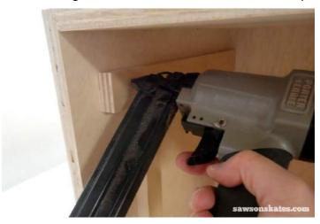
Hold the 13/16" scrap below the support, apply glue to another support, place below the scrap and attach using 1-1/4" brad nails. Remove the scrap.
