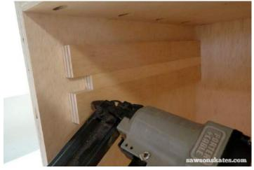
Place the 3-1/4" scrap on the bottom of the carcass, apply glue to a support, place on top of the scrap and attach using 1-1/4" brad nails. Remove the scrap.
