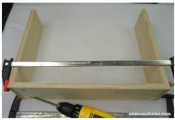
To make the drawer box fronts, rip two pieces of 3/4" plywood to 6" with a 5 degree bevel on one edge and cut to 19-3/8". Place the front in between the sides with 5 degree bevel on your workbench and mark the top edge of the front.
