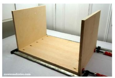
Attach using 1-1/4" pocket screws.
