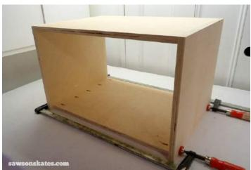
**Step 5.** Cut and Install the Back. Check the inside dimensions of your carcass. It should measure 22-1/2" x 13-1/8". Cut the back to fit the carcass from a piece of 3/4" plywood and drill pocket holes around the edges. Apply glue to the edges of the back, position in the carcass and attach using 1-1/4" pocket screws.
