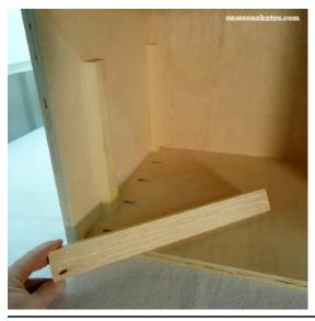
Attach using 1-1/4" brad nails. Remove the scrap.
