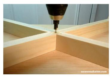
Attach using 2" wood screws.
