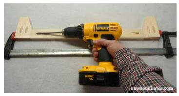
**Step 9.** Cut the Short Leg Braces. Cut two pieces of 1×2 to 9-5/16" with a 22.5 degree miter cut on one end. Drill a pocket hole on the opposite end of the miter. Apply glue to the end and attach a leg using 1-1/4" pocket screws.
