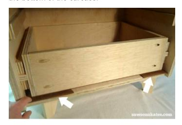
Place the drawer front on top of the scrap, then place 1/8" hardboard on each side and clamp in place. If you can't fit the 1/8" scrap on each side of the drawer front, adjust the length of the drawer front to fit.
