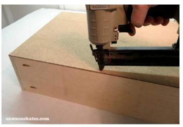
To make the drawer slides, rip 4 pieces of 3/4" plywood to 11/16" and cut to 15". Test fit the drawer slides and the drawer in the carcass. The drawer should move easily without being too loose – adjust the width of the slides if necessary. To install the drawer slide on the drawer box, place the drawer box on your workbench, clamp a scrap piece of 1 x3 to the side, place the slide on the scrap, mark the ends and cut to length.
