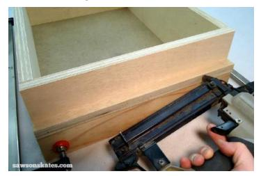
**Step 14.** Cut the Drawer Fronts and Attach to the Drawer Boxes. The drawer fronts attach to the drawer box and will be visible from the outside of the nightstand. Cut two pieces of 3/4" plywood to 22-1/4" x 7-1/2" (these pieces are cut a little wider than necessary in order to make the bevel cuts). Set your table saw to 5 degrees and cut a bevel on one side of each drawer front. From the beveled side measure 6-7/16" and cut a 5 degree bevel parallel to the first bevel.
