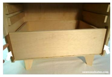
From inside the drawer box, drill countersink holes and attach using 1-1/4" wood screws.
