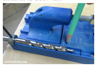
**Step 1.** Make the Top. Cut a piece of plywood to 22-1/2" x 16-1/2" and drill pocket holes in each end.
