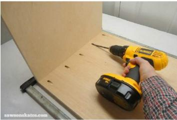
Apply glue to the bottom, clamp to the sides so that the bottom is flush with the back of the sides and attach using 1-1/4" pocket screws.
