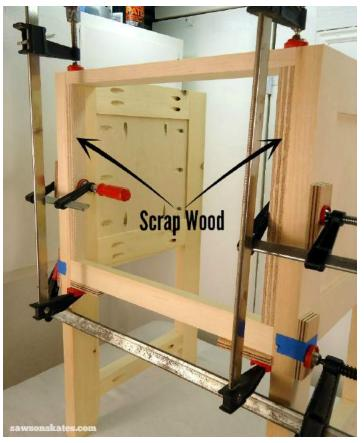
Slide the bottom in position. Make sure the bottom is flush with the bottom of the side rails and front rail. Clamp and attach using 1-1/4" pocket screws.
