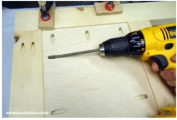
**Step 6.** Cut 5 pieces of 1×2 to 15-1/2" and drill a pocket hole in each end.
