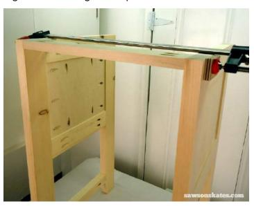
Apply glue to a 1×2 (from Step 6) and place 11-3/4" below the top brace. I cut a few pieces of scrap wood to 11-3/4" to help position this piece. Attach using 1-1/4" pocket screws.
