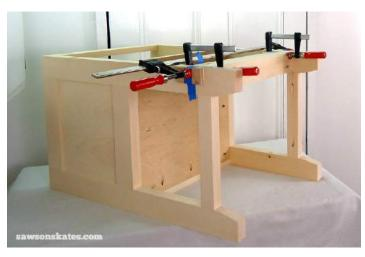
From the bottom, drill a countersink hole and attach using a 1-1/4" wood screw.
