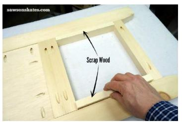
Once everything is laid out, apply glue to the ends of the rails, clamp the assembly and attach using 1-1/2" pocket screws. Do not attach the panel at this point.
