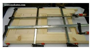
Flip the assembly over and be sure the panel sets in 1/4" from the face of the legs. Adjust if necessary. Clamp the panel in position, flip the assembly over and attach the panel with 1" pocket screws. Repeat for the other side.
